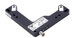
AutomationDirect photoelectric fork sensor, L-frame, die-cast zinc housing, through-beam, infrared light emission, 0-80mm sensing distance, 10-30 VDC operating voltage, selectable light-on/dark-on, PNP, 3-pin M8 quick-disconnect.
