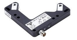
AutomationDirect photoelectric fork sensor, L-frame, die-cast zinc housing, through-beam, infrared, 0-60mm sensing distance, 10-30 VDC operating voltage, selectable light-on/dark-on, PNP, 3-pin M8 quick-disconnect.
