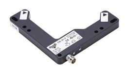
Photoelectric fork sensor, L-frame, through-beam, infrared light emission, 0-80mm sensing distance, selectable light-on/dark-on, NPN, potentiometer, 2 kHz switching frequency, die-cast zinc housing, 3-pin M8 quick-disconnect.
