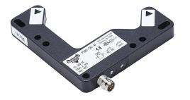
Photoelectric fork sensor, L-frame, through-beam, infrared light emission, 0-60mm sensing distance, selectable light-on/dark-on, NPN, potentiometer, 2 kHz switching frequency, die-cast zinc housing, 3-pin M8 quick-disconnect.
