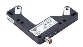
Photoelectric fork sensor, through-beam, 75 x 84 x 10mm, L-frame, infrared light emission, 0-60mm sensing distance, 10-30 VDC operating voltage, NPN, IP67, 3-pin M8 quick-disconnect.
