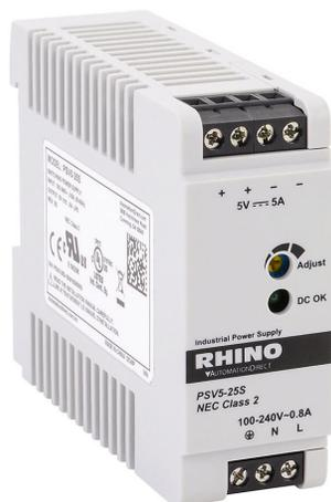
RHINO PSV series switching power supply, 5 VDC @ 5A/25W (adjustable), 120/240 VAC nominal input, 1-phase, enclosed, plastic housing, 35mm DIN rail mount, screw terminals, NEC Class 2.
