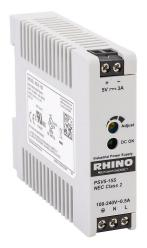
RHINO PSV series switching power supply, 5 VDC @ 3A/15W (adjustable), 120/240 VAC nominal input, 1-phase, enclosed, plastic housing, 35mm DIN rail mount, screw terminals, NEC Class 2.
