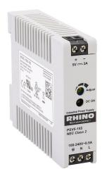
RHINO PSV series switching power supply, 5 VDC @ 3A/15W (adjustable), 120/240 VAC nominal input, 1-phase, enclosed, plastic housing, 35mm DIN rail mount, screw terminals, NEC Class 2.
