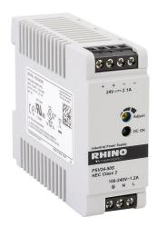
RHINO PSV series switching power supply, 24 VDC @ 2.1A/50W (adjustable), 120/240 VAC nominal input, 1-phase, enclosed, plastic housing, 35mm DIN rail mount, screw terminals, NEC Class 2.
