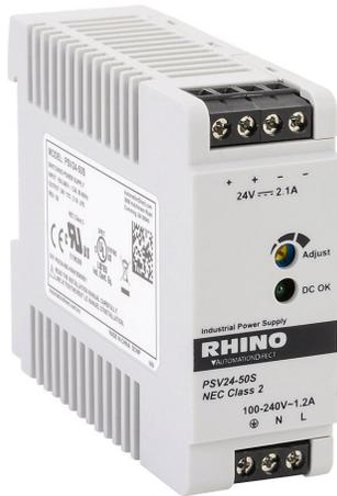
RHINO PSV series switching power supply, 24 VDC @ 2.1A/50W (adjustable), 120/240 VAC nominal input, 1-phase, enclosed, plastic housing, 35mm DIN rail mount, screw terminals, NEC Class 2.
