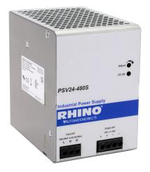
RHINO PSV series switching power supply, 24 VDC @ 20A/480W (adjustable), 120/240 VAC nominal input, 1-phase, enclosed, metal housing, 35mm DIN rail mount, screw terminals.
