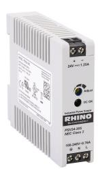
RHINO PSV series switching power supply, 24 VDC @ 1.25A/30W (adjustable), 120/240 VAC nominal input, 1-phase, enclosed, plastic housing, 35mm DIN rail mount, screw terminals, NEC Class 2.
