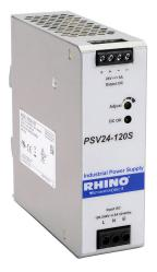
RHINO PSV series switching power supply, 24 VDC @ 5A/120W (adjustable), 120/240 VAC nominal input, 1-phase, enclosed, metal housing, 35mm DIN rail mount, screw terminals.
