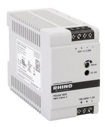
RHINO PSV series switching power supply, 24 VDC @ 3.8A/91W (adjustable), 120/240 VAC nominal input, 1-phase, enclosed, plastic housing, 35mm DIN rail mount, screw terminals, NEC Class 2.
