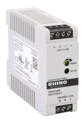
RHINO PSV series switching power supply, 12 VDC @ 4A/48W (adjustable), 120/240 VAC nominal input, 1-phase, enclosed, plastic housing, 35mm DIN rail mount, screw terminals, NEC Class 2.
