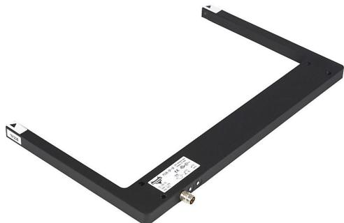
AutomationDirect photoelectric fork sensor, U-frame, die-cast zinc housing, through-beam, visible red, 0-220mm sensing distance, 10-30 VDC operating voltage, selectable light-on/dark-on, PNP, 3-pin M8 quick-disconnect.
