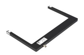
AutomationDirect photoelectric fork sensor, U-frame, die-cast zinc housing, through-beam, visible red, 0-220mm sensing distance, 10-30 VDC operating voltage, selectable light-on/dark-on, PNP, 3-pin M8 quick-disconnect.
