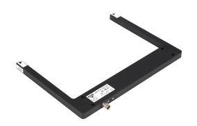
AutomationDirect photoelectric fork sensor, U-frame, die-cast zinc housing, through-beam, visible red, 0-180mm sensing distance, 10-30 VDC operating voltage, selectable light-on/dark-on, PNP, 3-pin M8 quick-disconnect.
