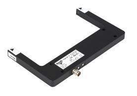
AutomationDirect photoelectric fork sensor, U-frame, die-cast zinc housing, through-beam, visible red, 0-120mm sensing distance, 10-30 VDC operating voltage, selectable light-on/dark-on, PNP, 3-pin M8 quick-disconnect.
