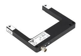
AutomationDirect photoelectric fork sensor, U-frame, die-cast zinc housing, through-beam, visible red, 0-80mm sensing distance, 10-30 VDC operating voltage, selectable light-on/dark-on, PNP, 3-pin M8 quick-disconnect.
