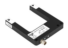
AutomationDirect photoelectric fork sensor, U-frame, die-cast zinc housing, through-beam, visible red, 0-50mm sensing distance, 10-30 VDC operating voltage, selectable light-on/dark-on, PNP, 3-pin M8 quick-disconnect.
