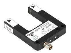
AutomationDirect photoelectric fork sensor, U-frame, die-cast zinc housing, through-beam, visible red, 0-30mm sensing distance, 10-30 VDC operating voltage, selectable light-on/dark-on, PNP, 3-pin M8 quick-disconnect.
