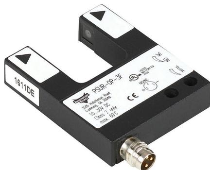
AutomationDirect photoelectric fork sensor, U-frame, die-cast zinc housing, through-beam, visible red, 0-20mm sensing distance, 10-30 VDC operating voltage, selectable light-on/dark-on, PNP, 3-pin M8 quick-disconnect.
