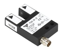
AutomationDirect photoelectric fork sensor, U-frame, die-cast zinc housing, through-beam, visible red, 0-10mm sensing distance, 10-30 VDC operating voltage, selectable light-on/dark-on, PNP, 3-pin M8 quick-disconnect.
