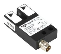
AutomationDirect photoelectric fork sensor, U-frame, die-cast zinc housing, through-beam, visible red light emission, 0-5mm sensing distance, 10-30 VDC operating voltage, selectable light-on/dark-on, PNP, 3-pin M8 quick-disconnect.
