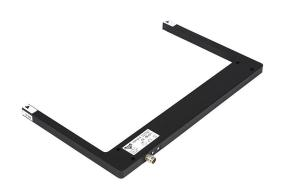
Photoelectric fork sensor, U-frame, through-beam, visible red light emission, 0-220mm sensing distance, selectable light-on/dark-on, NPN, potentiometer, 1.5 kHz switching frequency, diecast zinc housing, 3-pin M8 quick-disconnect.
