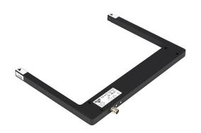
Photoelectric fork sensor, through-beam, 200 x 153 x 10mm, U-frame, visible red light emission, 0-180mm sensing distance, 10-30 VDC operating voltage, NPN, IP67, 3-pin M8 quick-disconnect.
