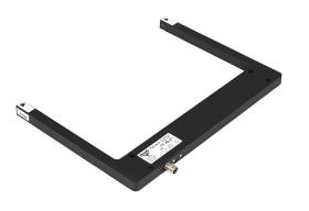
Photoelectric fork sensor, U-frame, through-beam, visible red light emission, 0-180mm sensing distance, selectable light-on/dark-on, NPN, potentiometer, 1.5 kHz switching frequency, diecast zinc housing, 3-pin M8 quick-disconnect.
