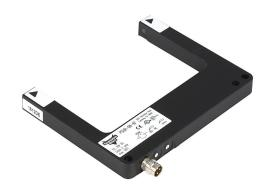
AutomationDirect photoelectric fork sensor, U-frame, die-cast zinc housing, through-beam, visible red light emission, 0-80mm sensing distance, 10-30 VDC operating voltage, selectable light-on/dark-on, NPN, 3-pin M8 quick-disconnect.
