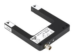
AutomationDirect photoelectric fork sensor, U-frame, die-cast zinc housing, through-beam, visible red, 0-50mm sensing distance, 10-30 VDC operating voltage, selectable light-on/dark-on, NPN, 3-pin M8 quick-disconnect.
