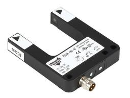
AutomationDirect photoelectric fork sensor, U-frame, die-cast zinc housing, through-beam, visible red, 0-30mm sensing distance, 10-30 VDC operating voltage, selectable light-on/dark-on, NPN, 3-pin M8 quick-disconnect.
