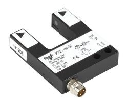
AutomationDirect photoelectric fork sensor, U-frame, die-cast zinc housing, through-beam, visible red, 0-20mm sensing distance, 10-30 VDC operating voltage, selectable light-on/dark-on, NPN, 3-pin M8 quick-disconnect.
