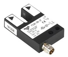
AutomationDirect photoelectric fork sensor, U-frame, die-cast zinc housing, through-beam, visible red, 0-10mm sensing distance, 10-30 VDC operating voltage, selectable light-on/dark-on, NPN, 3-pin M8 quick-disconnect.
