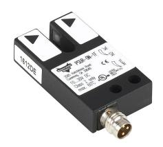
AutomationDirect photoelectric fork sensor, U-frame, die-cast zinc housing, through-beam, visible red, 0-5mm sensing distance, 10-30 VDC operating voltage, selectable light-on/dark-on, NPN, 3-pin M8 quick-disconnect.
