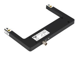
AutomationDirect photoelectric fork sensor, U-frame, die-cast zinc housing, through-beam, Class 1 red laser, 0-120mm sensing distance, 10-30 VDC operating voltage, selectable light-on/dark-on, PNP, 3-pin M8 quick-disconnect.
