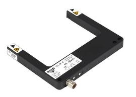
AutomationDirect photoelectric fork sensor, U-frame, die-cast zinc housing, through-beam, Class 1 red laser, 0-80mm sensing distance, 10-30 VDC operating voltage, selectable light-on/dark-on, PNP, 3-pin M8 quick-disconnect.
