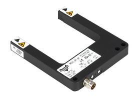
AutomationDirect photoelectric fork sensor, U-frame, die-cast zinc housing, through-beam, Class 1 red laser, 0-50mm sensing distance, 10-30 VDC operating voltage, selectable light-on/dark-on, PNP, 3-pin M8 quick-disconnect.
