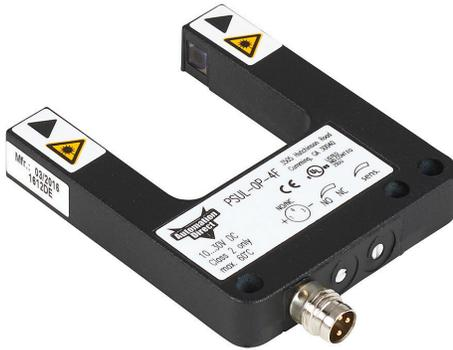
AutomationDirect photoelectric fork sensor, U-frame, die-cast zinc housing, through-beam, Class 1 red laser, 0-30mm sensing distance, 10-30 VDC operating voltage, selectable light-on/dark-on, PNP, 3-pin M8 quick-disconnect.
