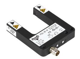
AutomationDirect photoelectric fork sensor, U-frame, die-cast zinc housing, through-beam, Class 1 laser light emission, 0-30mm sensing distance, 10-30 VDC operating voltage, selectable light-on/dark-on, PNP, 3-pin M8 quick-disconnect.
