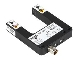
AutomationDirect photoelectric fork sensor, U-frame, die-cast zinc housing, through-beam, Class 1 red laser, 0-30mm sensing distance, 10-30 VDC operating voltage, selectable light-on/dark-on, PNP, 3-pin M8 quick-disconnect.
