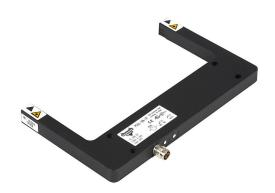
AutomationDirect photoelectric fork sensor, U-frame, die-cast zinc housing, through-beam, Class 1 red laser, 0-120mm sensing distance, 10-30 VDC operating voltage, selectable light-on/dark-on, NPN, 3-pin M8 quick-disconnect.
