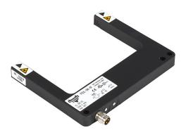
AutomationDirect photoelectric fork sensor, U-frame, die-cast zinc housing, through-beam, Class 1 red laser, 0-80mm sensing distance, 10-30 VDC operating voltage, selectable light-on/dark-on, NPN, 3-pin M8 quick-disconnect.
