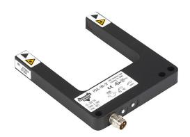
AutomationDirect photoelectric fork sensor, U-frame, die-cast zinc housing, through-beam, Class 1 laser light emission, 0-50mm sensing distance, 10-30 VDC operating voltage, selectable light-on/dark-on, NPN, 3-pin M8 quick-disconnect.
