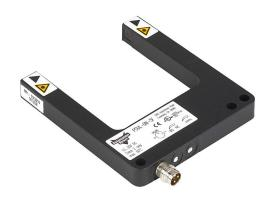
AutomationDirect photoelectric fork sensor, U-frame, die-cast zinc housing, through-beam, Class 1 red laser, 0-50mm sensing distance, 10-30 VDC operating voltage, selectable light-on/dark-on, NPN, 3-pin M8 quick-disconnect.
