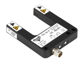
AutomationDirect photoelectric fork sensor, U-frame, die-cast zinc housing, through-beam, Class 1 laser light emission, 0-30mm sensing distance, 10-30 VDC operating voltage, selectable light-on/dark-on, NPN, 3-pin M8 quick-disconnect.
