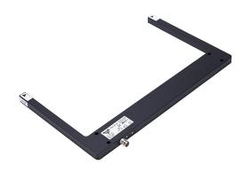
AutomationDirect photoelectric fork sensor, U-frame, die-cast zinc housing, through-beam, infrared light emission, 0-220mm sensing distance, 10-30 VDC operating voltage, selectable light-on/dark-on, PNP, 3-pin M8 quick-disconnect.
