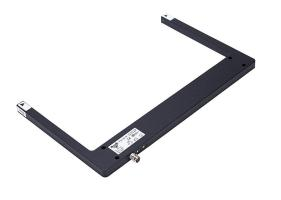
AutomationDirect photoelectric fork sensor, U-frame, die-cast zinc housing, through-beam, infrared, 0-220mm sensing distance, 10-30 VDC operating voltage, selectable light-on/dark-on, PNP, 3-pin M8 quick-disconnect.
