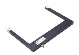
AutomationDirect photoelectric fork sensor, U-frame, die-cast zinc housing, through-beam, infrared, 0-180mm sensing distance, 10-30 VDC operating voltage, selectable light-on/dark-on, PNP, 3-pin M8 quick-disconnect.
