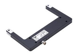
AutomationDirect photoelectric fork sensor, U-frame, die-cast zinc housing, through-beam, infrared light emission, 0-120mm sensing distance, 10-30 VDC operating voltage, selectable light-on/dark-on, PNP, 3-pin M8 quick-disconnect.
