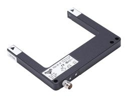
AutomationDirect photoelectric fork sensor, U-frame, die-cast zinc housing, through-beam, infrared, 0-80mm sensing distance, 10-30 VDC operating voltage, selectable light-on/dark-on, PNP, 3-pin M8 quick-disconnect.
