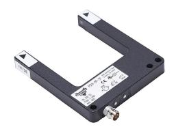
AutomationDirect photoelectric fork sensor, U-frame, die-cast zinc housing, through-beam, infrared light emission, 0-50mm sensing distance, 10-30 VDC operating voltage, selectable light-on/dark-on, PNP, 3-pin M8 quick-disconnect.
