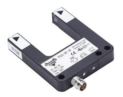
AutomationDirect photoelectric fork sensor, U-frame, die-cast zinc housing, through-beam, infrared light emission, 0-30mm sensing distance, 10-30 VDC operating voltage, selectable light-on/dark-on, PNP, 3-pin M8 quick-disconnect.
