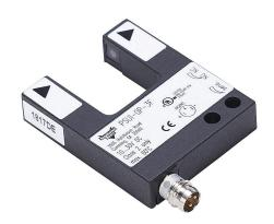
AutomationDirect photoelectric fork sensor, U-frame, die-cast zinc housing, through-beam, infrared, 0-20mm sensing distance, 10-30 VDC operating voltage, selectable light-on/dark-on, PNP, 3-pin M8 quick-disconnect.
