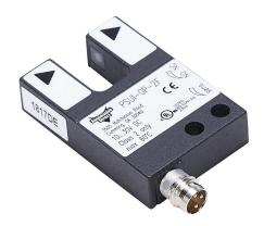
AutomationDirect photoelectric fork sensor, U-frame, die-cast zinc housing, through-beam, infrared, 0-10mm sensing distance, 10-30 VDC operating voltage, selectable light-on/dark-on, PNP, 3-pin M8 quick-disconnect.
