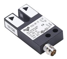
AutomationDirect photoelectric fork sensor, U-frame, die-cast zinc housing, through-beam, infrared, 0-5mm sensing distance, 10-30 VDC operating voltage, selectable light-on/dark-on, PNP, 3-pin M8 quick-disconnect.
