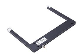
Photoelectric fork sensor, through-beam, 200 x 153 x 10mm, U-frame, infrared light emission, 0-180mm sensing distance, 10-30 VDC operating voltage, NPN, IP67, 3-pin M8 quick-disconnect.
