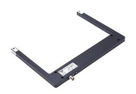
Photoelectric fork sensor, U-frame, through-beam, infrared light emission, 0-180mm sensing distance, selectable light-on/dark-on, NPN, potentiometer, 2 kHz switching frequency, die-cast zinc housing, 3-pin M8 quick-disconnect.
