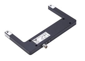
Photoelectric fork sensor, U-frame, through-beam, infrared light emission, 0-120mm sensing distance, selectable light-on/dark-on, NPN, potentiometer, 1 kHz switching frequency, die-cast zinc housing, 3-pin M8 quick-disconnect.
