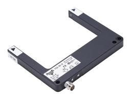
AutomationDirect photoelectric fork sensor, U-frame, die-cast zinc housing, through-beam, infrared, 0-80mm sensing distance, 10-30 VDC operating voltage, selectable light-on/dark-on, NPN, 3-pin M8 quick-disconnect.
