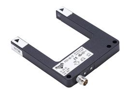
AutomationDirect photoelectric fork sensor, U-frame, die-cast zinc housing, through-beam, infrared, 0-50mm sensing distance, 10-30 VDC operating voltage, selectable light-on/dark-on, NPN, 3-pin M8 quick-disconnect.
